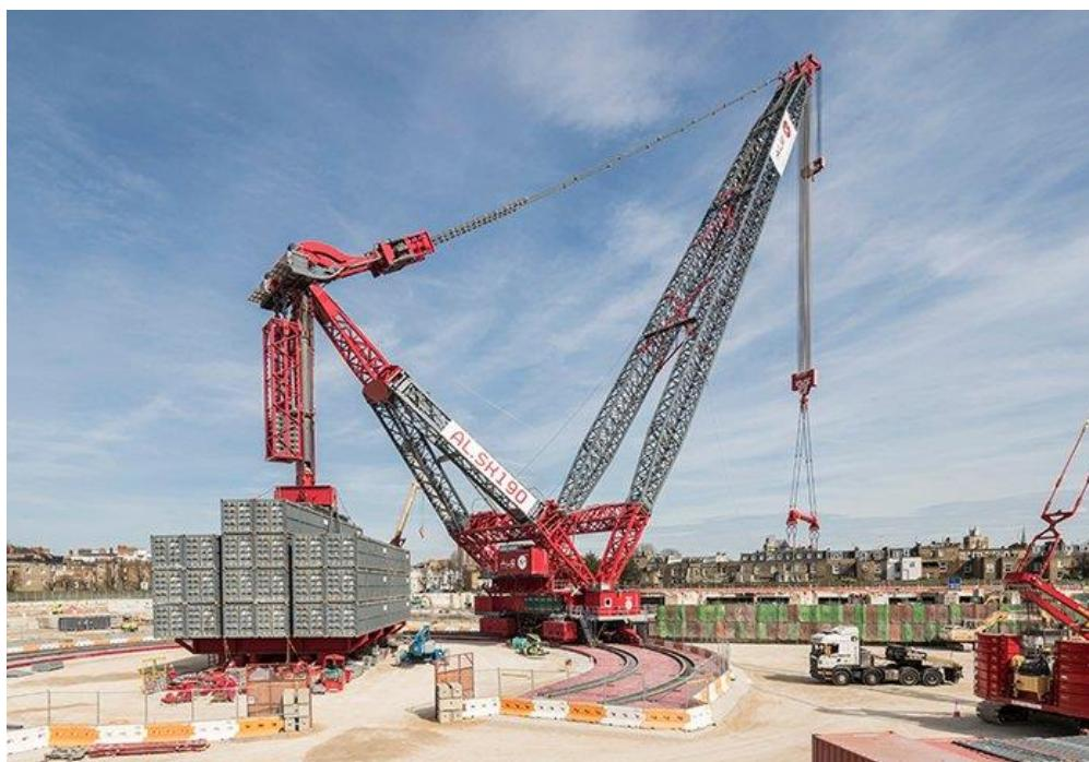
Slika 3.2. Kranska dizalica AL.SK nosivosti 4300 tona na trakastom temeljnem nosaču; Izvor: <https://www.ale-heavylift.com/knowledge-centre/case-studies/lifting-portal-beams-with-the-al-sk190-at-earls-court-uk/>
