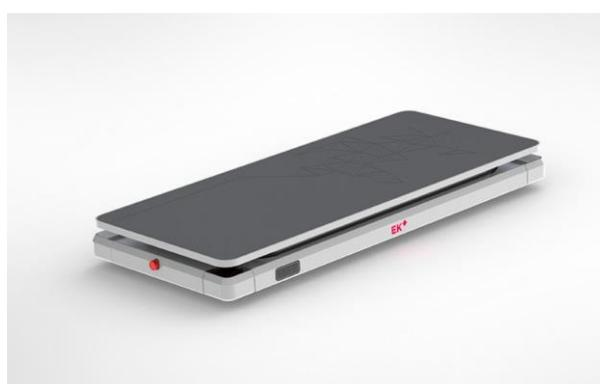
*Slika 40. Ultra ravan transportni robot FAST MOVE*
