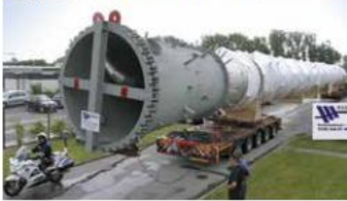
Hydrolyser column in duplex stainless steel.
