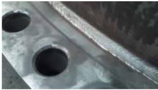
Flange welded with TETRA S 22 9 3L-G.
