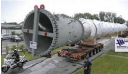
Hydrolyser column in duplex stainless steel.
