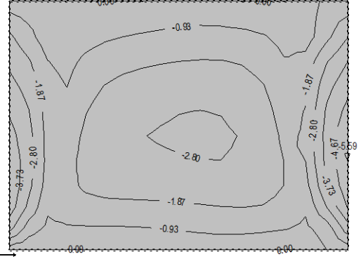
Okvir: V_3 Aa - g.zona - Pramac 1 - max Aa1,g= -5.59 cm 2 /m
