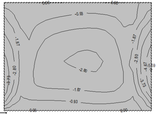
Okvir: V_3 Aa - g.zona - Pramac 1 - max Aa1,g= -5.59 cm²/m
