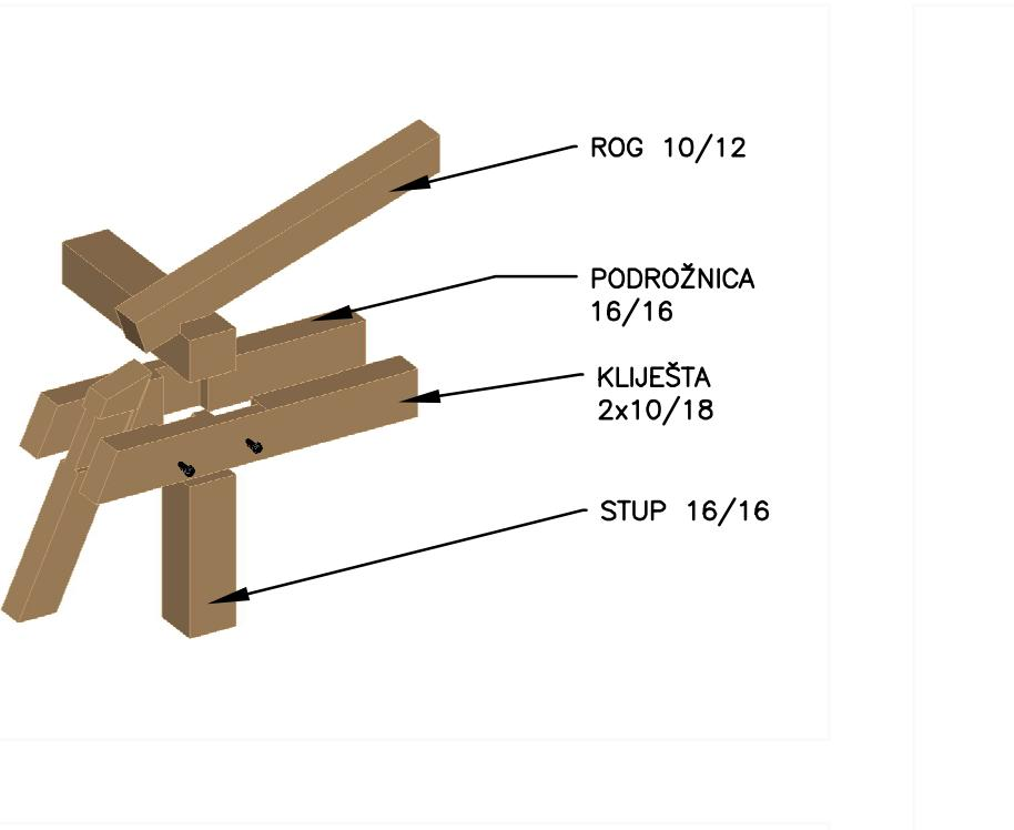
PRIKAZ JEDOSTREŠNOG MANSARDNOG KROVIŠTA S JEDNOSTRUKOM VISULJOM M 1:50
