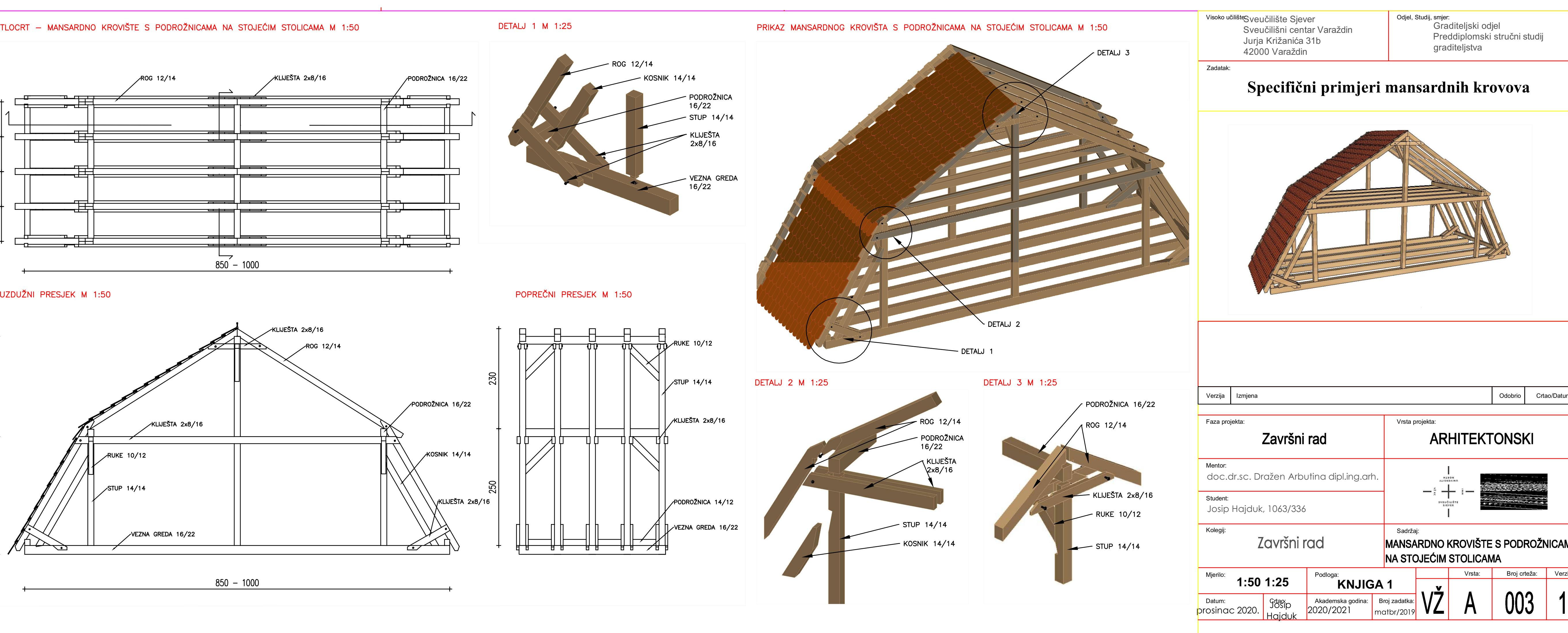
TLOCRT – MANSARDNO KROVIŠTE OD LAMELIRANOG DRVA M 1:50
