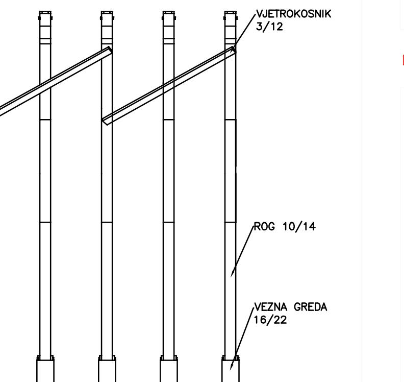
PRIKAZ MANSARDNOG KROVIŠTA OD LAMELIRANOG DRVA M 1:50
