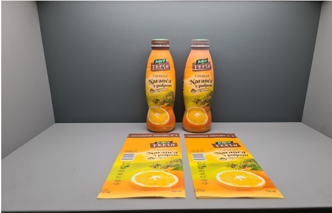
Slika 6.2 600 mm 18 Watt VeriVide Artificial Daylight D65
