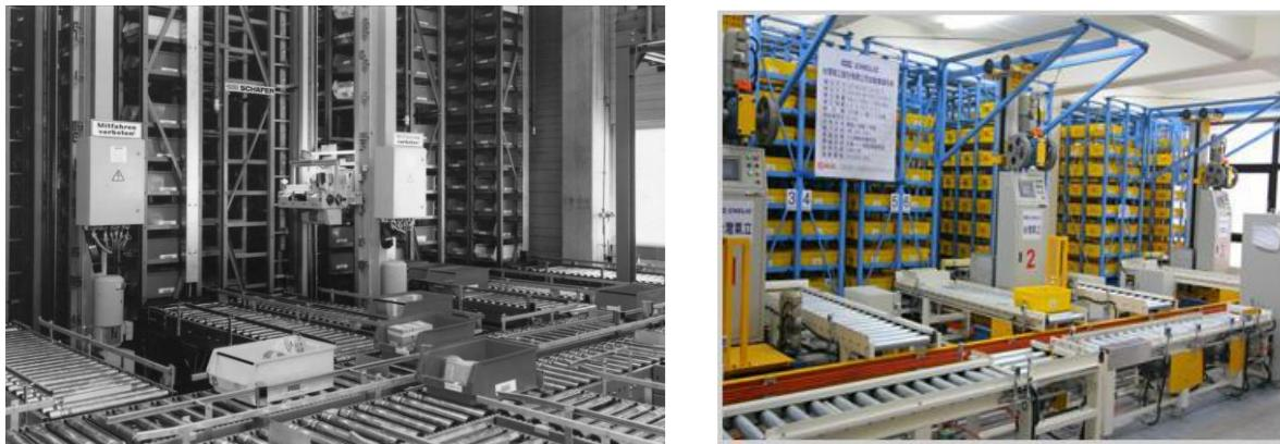
*Slika 3.5 Mini-load i Micro-Load AS/RS sustav [6]*
