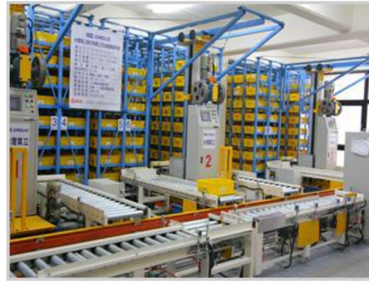
Slika 3.5 Mini-load i Micro-Load AS/RS sustav [6]
