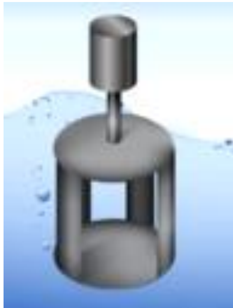
Slika 2.8. Squirrel cage Darrieus turbina [4]
