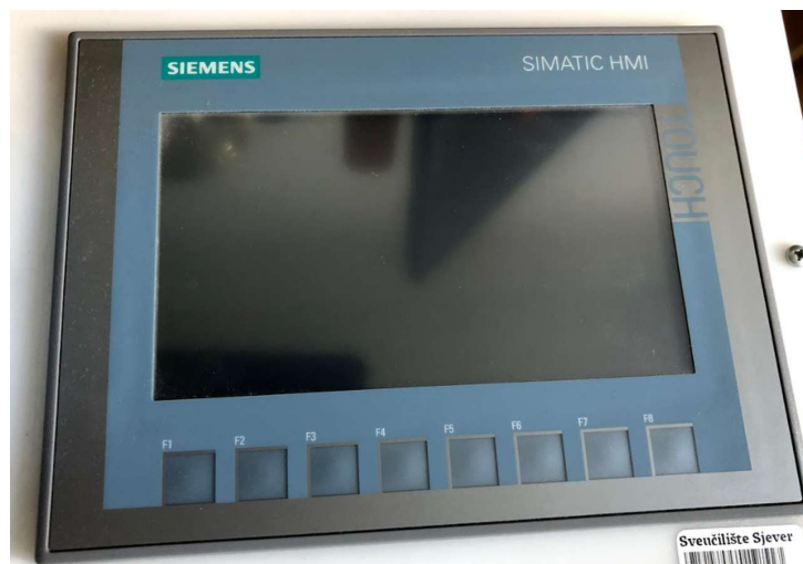
Slika 4. 2 Korišten HMI panel KTP700 Basic PN
