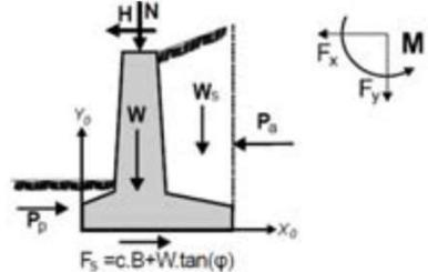
$$\text{Trenje tla } Rd=N_d \cdot \tan(\phi/\gamma M)= 75,231 \text{ kN/m}'$$
