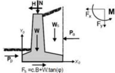
$$\text{Trenje tla} \quad R_d = N_d \cdot \tan(\phi / \gamma M) = 64,470 \text{ kN/m}'$$
