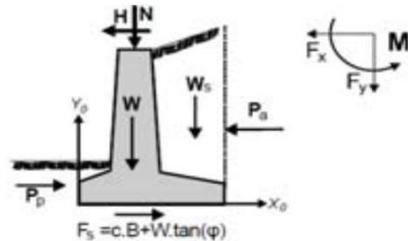
$$\text{Trenje tla } Rd = Nd \cdot \tan(\phi) / \gamma M = 58,023 \text{ kN/m'}$$
