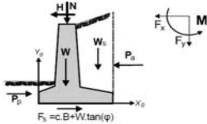
$$\text{Trenje tla} \quad R_d = N_d \cdot \tan(\phi) / \gamma M = 55,331 \text{ kN/m}'$$
