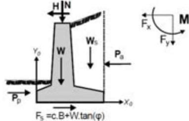
$$\text{Trenje tla } Rd=N_d \cdot \tan(\phi/\gamma M)= 71,741 \text{ kN/m}'$$
