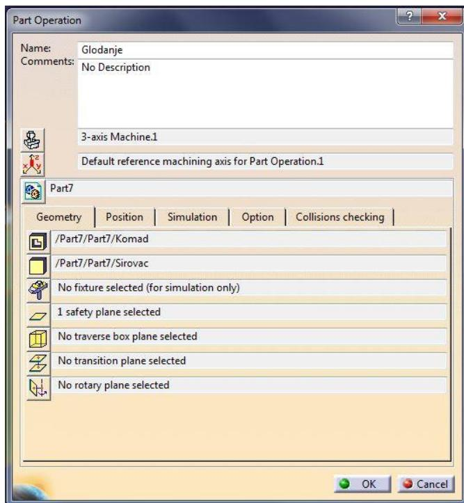
**Slika 5.2.2 Odabir kalupa i sirovca [3]**
