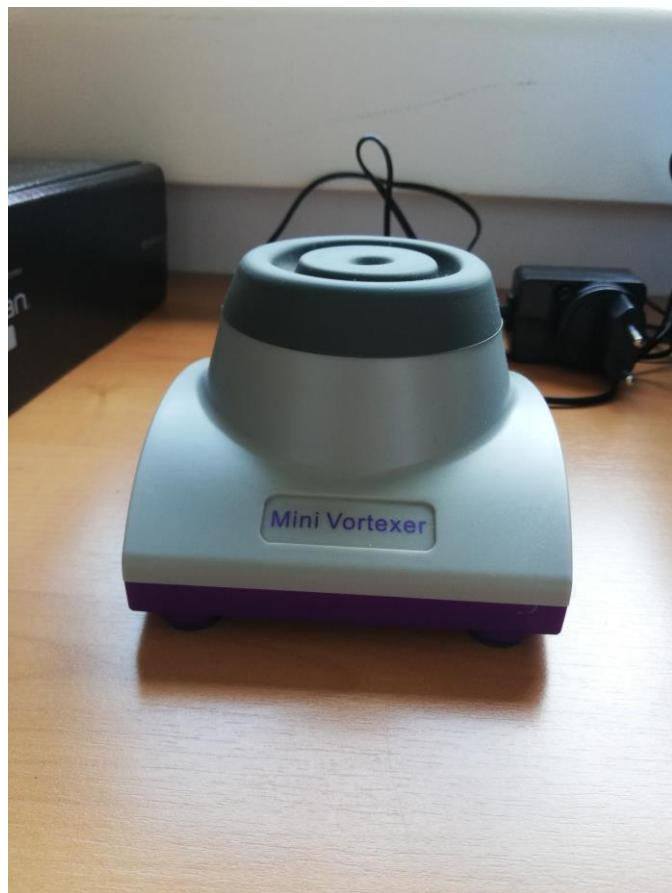
Slika 11. Mini Vortexer homogenizator, Heathrow Scientific, Kina
