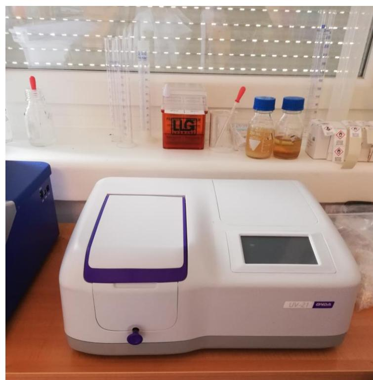
*Slika 9. spektrofotometar, UV/Visible Spectrophotometer 195-1050 nm, 4 nm bandwith,
