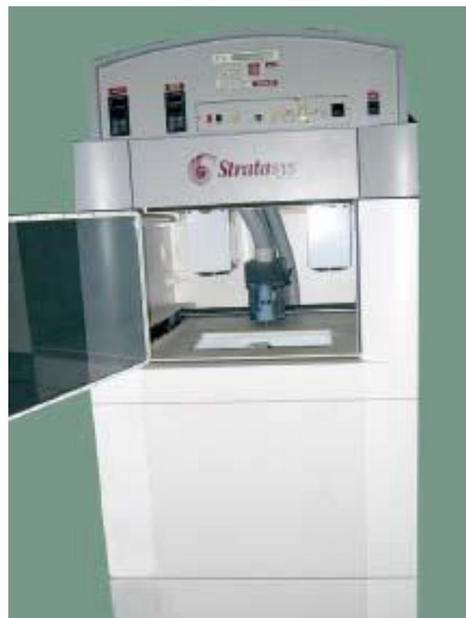
Slika 1.1 Prvi FDM 3D printer (Stratasys 3D Modeler)[1]
