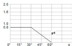
$$S(\alpha_1) = \mu_1(\alpha_1) \cdot C_e \cdot C_t \cdot S_k = 0.400 \times 1.000 \times 1.000 \times 1.300 = 0.520 \text{ kN/m}^2$$
