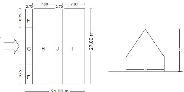
Zone : F,  $A = 25.77 \text{ m}^2$ ,  $C_{pe,10} = +0.70$ ,  $C_{pe,1} = +0.70$
