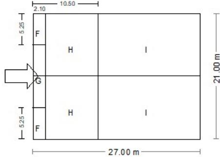
Zone : F,  $A = 15.59 \text{ m}^2$ ,  $C_{pe,10} = -1.10$ ,  $C_{pe,1} = -1.50$
