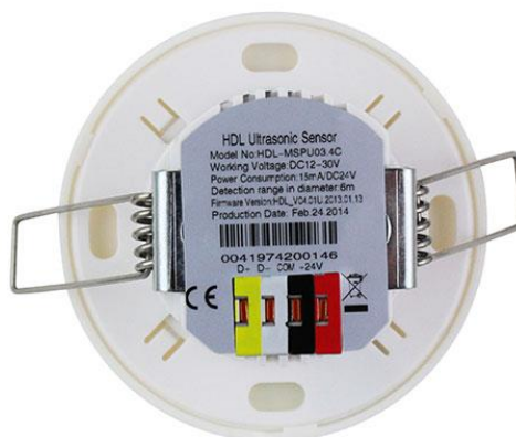
Slika 2.14. Ceiling Mount Ultrasonic Sensor [20]
