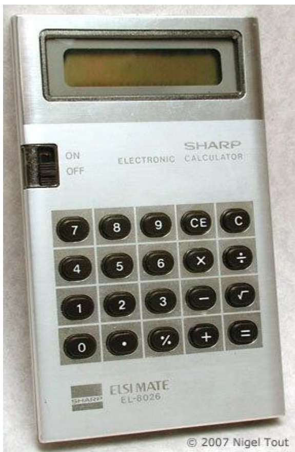
Slika 2.4 Prvi solarni kalkulator Sharp EL-8026 sprijeda ( http://www.vintagecalculators.com/assets/images/SharpEL8026_1.jpg )
