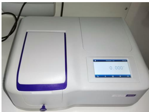
Slika 12: Spektrofotometar, UV/Visible Spectrophotometer 195-1050 nm, 4 nm bandwidth, Italija
