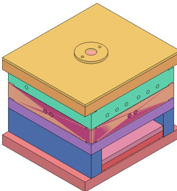
Slika 4.6.9.2. 3D model kalupa u CAD programu [22]
