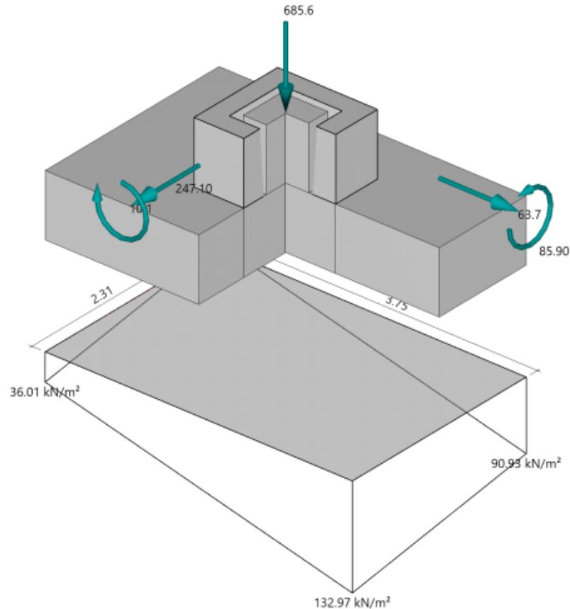
Bearing pressure figure without Self-weight
