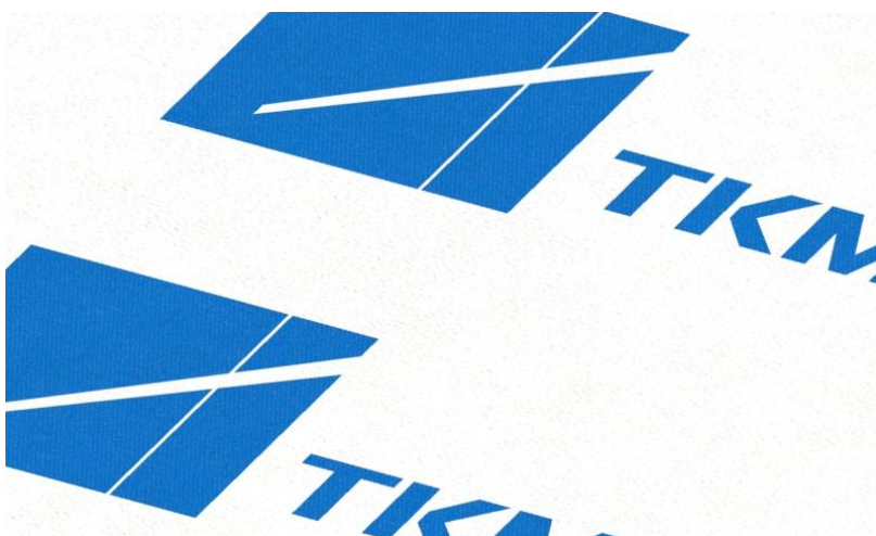
Slika 41. Negative doctor blade lines
