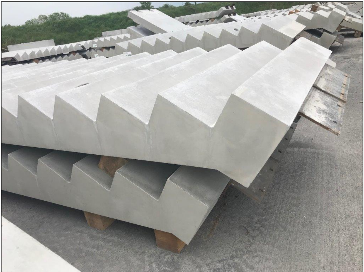
Slika 34: Odlaganje prefabriciranih stubišnih krakova (izvor: https://floodprecast.co.uk/2020/01/benefits-of-using-precast-stairs-with-steel-frame-buildings/ )
