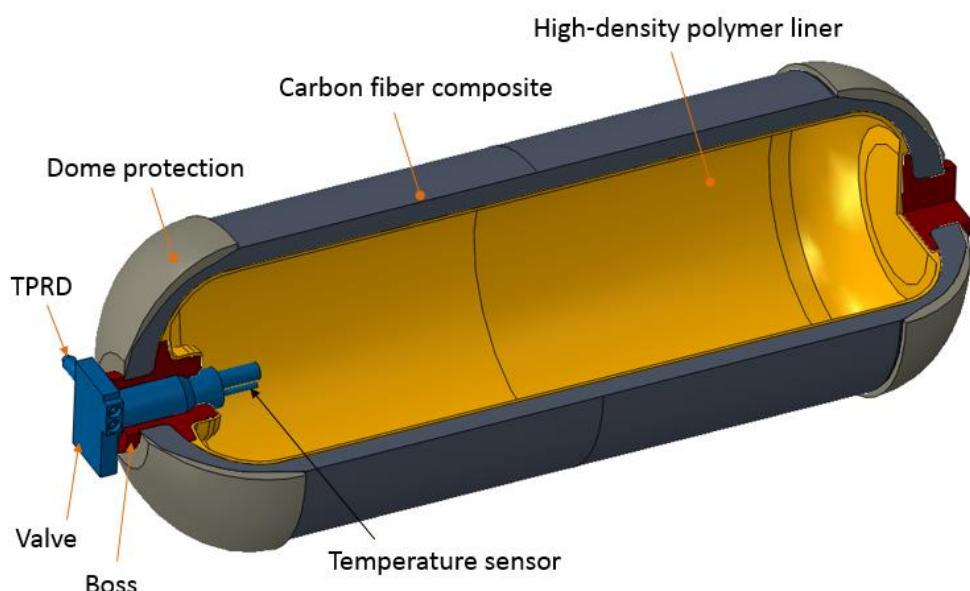
TPRD = Thermally Activated Pressure Relief Device
