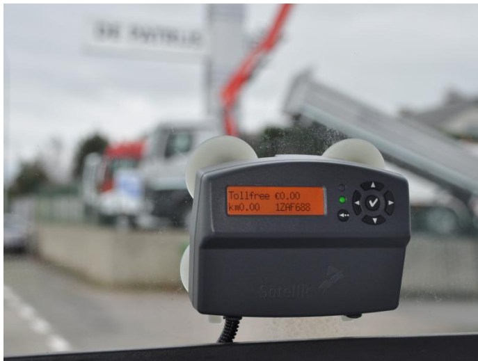
Slika 41 On Board Unit (OBU)
