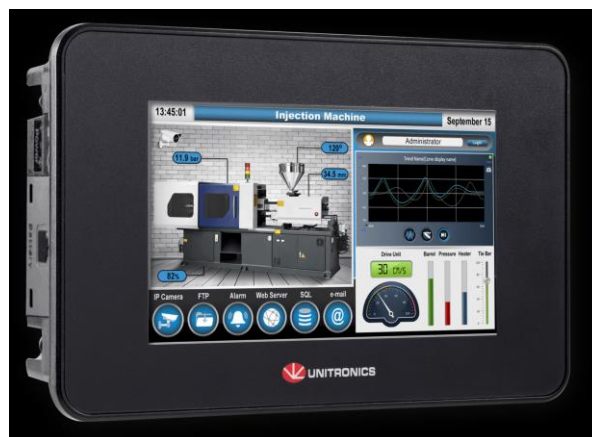
Slika 5.1. PLC UNITRONICS US5 – B10 – RA28
