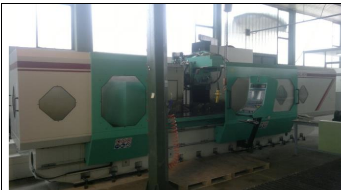
Slika 4.12 CNC brusilica Rosa – Linear Silver 30.8
